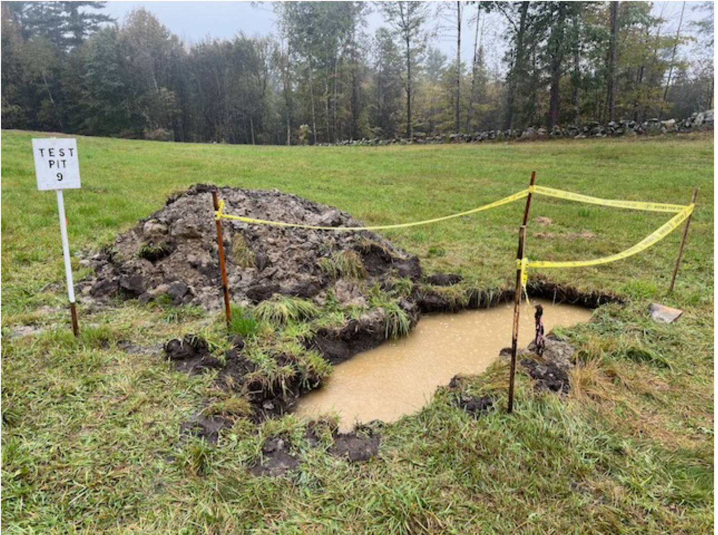
“After” prolonged heavy rains, photo of TP-9. Note absence of rock fragments in the backdirt pile, while a prominent stone wall is seen in the background. The transition to till parent material is ~ 80 feet to the left of the soil pit, at the slope break seen in the previous photo.
