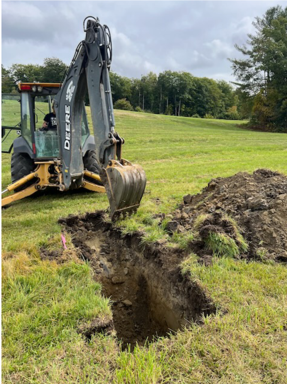
“Before” (dry season) TP-9 at the Berry Road farmland. The soil pit was dug during a prolonged dry period. The slope break in the background indicates the transition to lodgement tills. The hillside was formerly prime beach front property during deglaciation.
